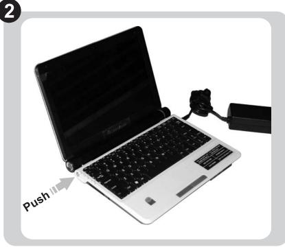
Connect the supplied DC Jack to the product. Push the Power button to turn on the laptop
