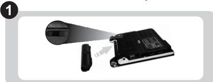
Ensure the battery is properly locked in place as shown.
